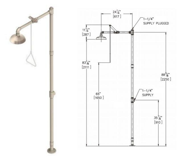
Model S2300-AS is our stainless steel free standing emergency shower, complete with stainless steel shower head. Complete with a 1" stainless steel stay open shower ball valve and is supplied with a safety sign and weekly testing card.
